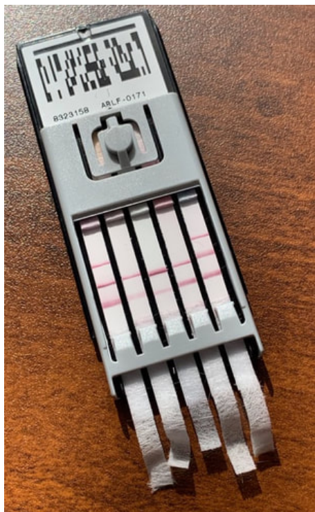
Figure 8 - The inside of the STK showing the analytical strips used to determine the presence of the tested-for substances. The red bands are only visible when a reading is obtained
