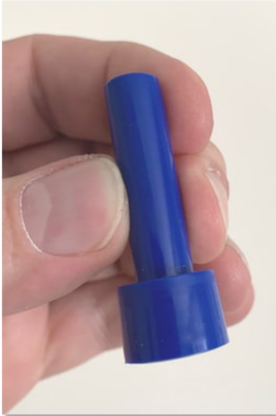
Figure 10 - The blue cap contained liquid used for an immunoassay colorimetric test carried out within the Dräger 5000.
